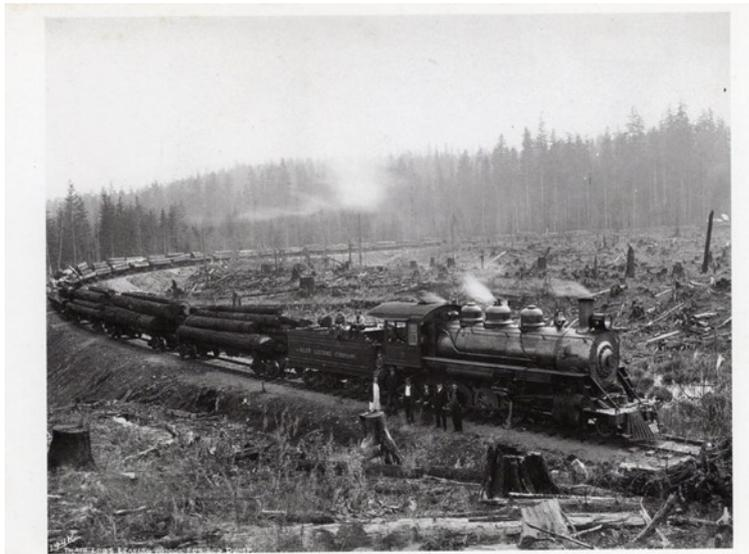
Pulling a large train of logs, this 2-8-2 steam locomotive is a Mikado built by the American company Baldwin Locomotive Works and owned by the Siler Logging Company in 1924.
