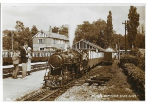
The railway is probably best known for its superb fleet of one-third full size steam and diesel locomotives, all of which have been built to run safely at speeds up to 25mph on rails only 15" apart.
